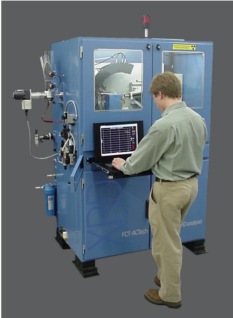
Figure 6: COSMA is designed for fully automated operation, but can be used for single sample analysis through the local operator interface. An internet connection allows for remote support and troubleshooting.
